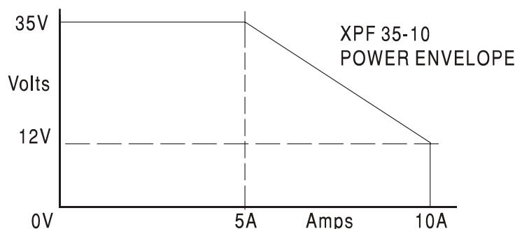
The power envelope is set to give 35V/5A and 12V/10A under all supply conditions (both outputs loaded); at lower output voltages the output power is restricted by the 10A current maximum.
