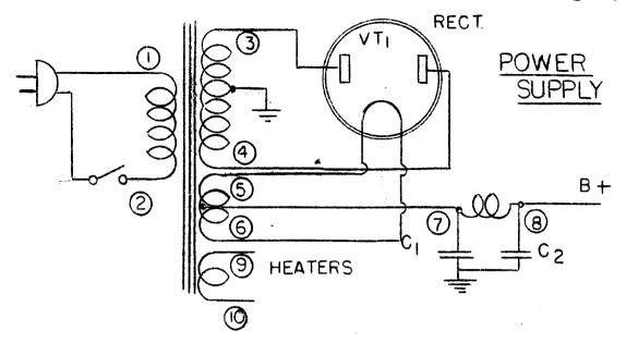
POWER SUPPLY SECTION: Since the audio frequency section has a blocking condenser in its input it will neglect any D.C. voltage and therefore it can be used to measure A.C. voltage irrespective of whether or not they have a D.C. component superimposed upon the A.C.
