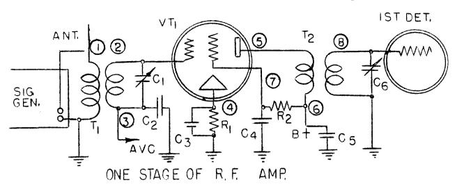
R.F. AMPLIFIER: The signal generator is connected in at antenna post 1 and ground.
