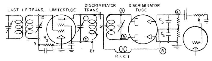
SECOND DETECTOR OF FREQUENCY MODULATED RECEIVERS: It will be noted that the second detector of frequency modulated receivers correspond almost identically to the circuit used for obtaining automatic frequency control voltage in amplitude modulated receivers, the exception being that the output of the discriminator tube at Point 6 instead of going directly to the grid of the control tube goes through a condenser and then to the first audio frequency amplifier.
