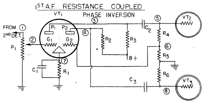
FIRST AUDIO FREQUENCY AMPLIFIER STAGE INVERTED: The signal supplied to the first audio frequency amplifier can either be fed directly in as audio frequency at point 1, which is the high end of the volume control, or can be fed in thru the antenna in the conventional manner with the 400 cycle modulated RF signal and the receiver tuned for the proper frequency being generated by the signal generator.
