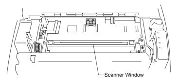
Fig. 5-22 Cleaning the Scanner Window
