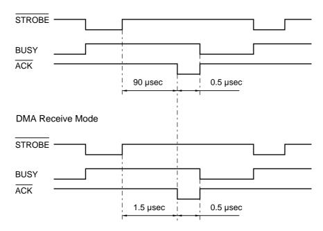
BUSY goes HIGH at the falling edge of the STROBE signal. The data (8 bits) from the PC is latched into the data buffer at the rising edge of the STROBE signal. The pulse width of ACK varies according to the speed MODE as shown above. BUSY goes LOW on the rising edge of ACK.
