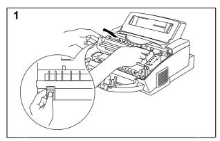
Open the top cover towards you. Remove the drum unit by holding each side of the drum and gently lifting the drum forwards towards you.
