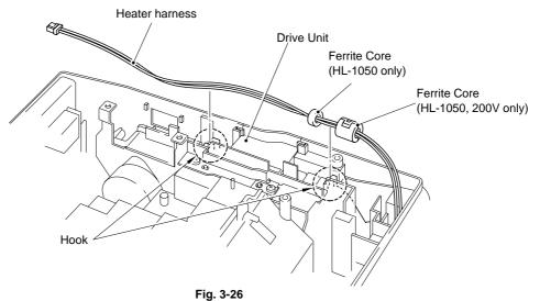
(2) Remove the three M4x20 and one M4x12 screws securing the drive unit.
