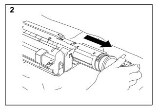
Remove the toner cartridge from the drum unit and keep it in a safe place.
