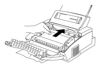
Fig. 6-6 Paper Jam Inside the Printer
