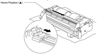
Fig. 5-23 Cleaning the Primary Corona Wire
