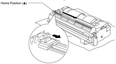
Fig. 5-9 Cleaning the Primary Corona Wire
