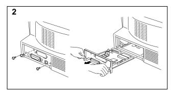
Unscrew the screws securing the rear plate of the main controller board to the printer and pull out the main controller board.
