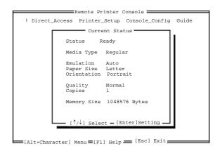
The RPC gets the current settings information from your printer when it starts if bi-directional communication is enabled between your computer and printer. Otherwise, RPC shows its default settings. If you want to change settings, move the cursor to the desired item and select the desired setting by using the **Enter** and **cursor** keys. Then, press the **Enter** key to make the selected setting valid. If you use a mouse, click the desired item to change the setting.
