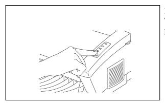
Press the control panel **switch**. The printer will start printing a test sample page.
