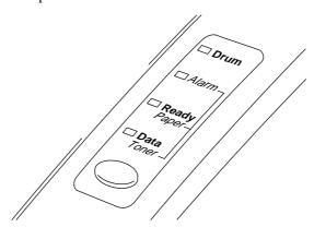
Fig. 3-1 Lamps and Switch on Control Panel
