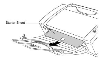
Fig. 5-18 Ejecting the Starter Sheet
