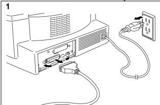
Turn off the **power** switch and unplug the p cord from the AC outlet. Disconnect the inte cable (printer cable) from the printer.
