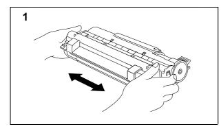
Unpack the drum unit assembly with the toner cartridge included. Gently shake it from side to side five or six times.
