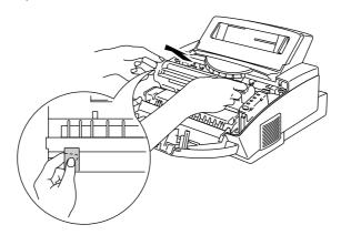
Fig. 5-2 Removing the Drum Unit
