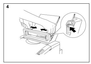
Hold the tab of the right hand paper guide and press the catch to release the guide lock. Move the paper guide to fit the paper width.
