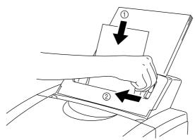
Fig. 2-7 Moving the Paper Guide
