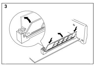
Install the SIMM into the slot and push it gently towards the vertical until it clicks into place.
