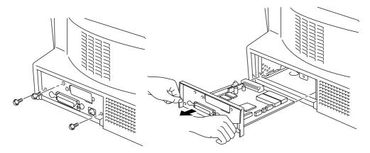
Fig. 4-4 Removing the Main Controller Board
