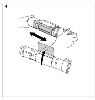
Unpack the new toner cartridge, gently shake it five or six times and then remove the protective part.
