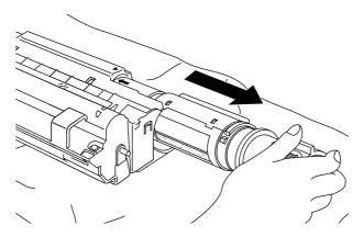
Fig. 5-5 Removing the Old Toner Cartridge
