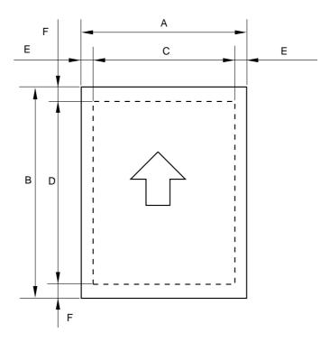
The effective printing area means the area within which the printing of all the data received without any omissions can be guaranteed.
