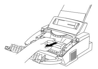
Fig. 6-5 Paper Jam near the Drum Unit
