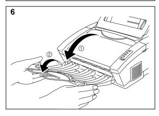
Open the output tray. (1) Extend the extension support wire. (2)
