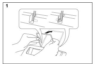
Install the paper support onto the multipurpose sheet feeder.
