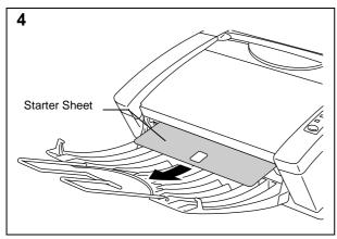
Make sure that the printer automatically ejects the starter sheet while the printer is warming-up immediately after installing a new drum unit.
