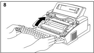
Re-install the drum unit into the printer and close the top cover.
