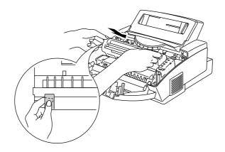
Fig. 5-17 Installing the Drum Unit
