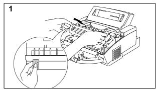
Open the top cover towards you. Remove the drum unit by holding each side of the drum and gently lifting the drum forwards towards you.
