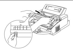
Fig. 5-24 Removing the Drum Unit Assembly
