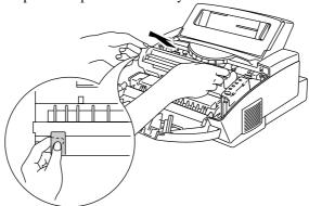
Fig. 5-12 Removing the Drum Unit
