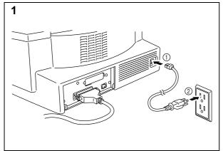
Plug the power cord into the AC power outlet and the printer power inlet.
