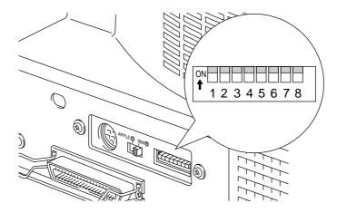
Fig. 4-2 Setting the Serial Interface Parameters
