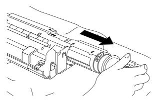
Fig. 5-14 Removing the Toner Cartridge
