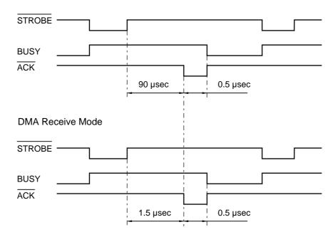
BUSY goes HIGH at the falling edge of STROBE. The data (8 bits) from the PC is latched in the data buffer at the rising edge of STROBE. The pulse width of ACK differs according to the speed MODE as shown above. BUSY goes LOW at the rising edge of ACK.
