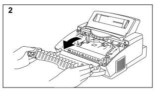
Open the top cover of the printer by holding both sides of it.
