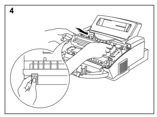
Install the toner cartridge into the new drum unit.
