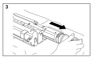
Remove the old toner cartridge from the drum unit by pulling it out gently.
