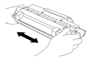
Fig. 5-15 Shaking the Drum Unit
