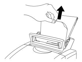
Fig. 6-4 Paper Jam in the Feeder
