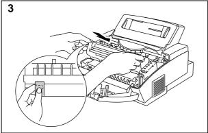
Holding the drum by its handles, install it into the printer.
