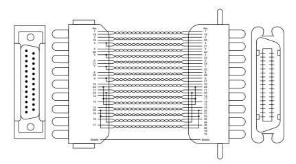
Fig. A-1 Parallel Interface Cable
