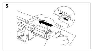
Install the new toner cartridge into the right hand side of the drum unit. Make sure that the toner cartridge guide bar is exactly aligned with the guide slot in the drum unit and pushed fully home into the drum unit to ensure that the toner cartridge and the drum unit fit together correctly.
