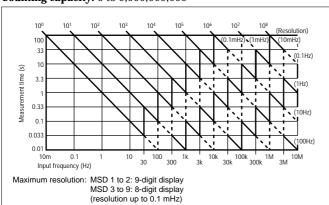
Fig. 1 Measurement Time, Resolution and Number of Periods With Respect To Input Frequency
