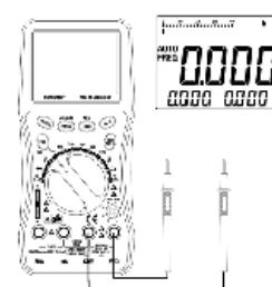
Connect the black measuring line to the COM socket (14) and the red measuring line to the VΩ socket (13) until these come to flatly lie on the measuring instrument.
