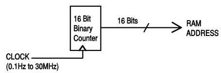
Arbitrary waveforms have a user defined length of 4 to 65536 points. Squarewaves use a fixed length of 2 points and pulse and pulse train have their length defined by the user selected period value.
