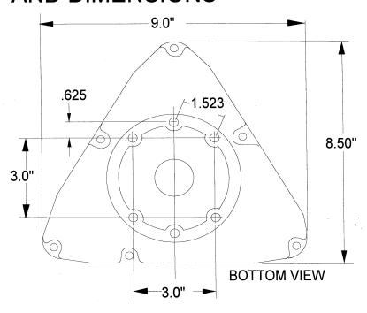
NOTE: FOR MAST DIAMETERS OVER 2-1/2" CONTACT M2 FOR LONGER BOLTS
