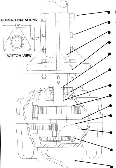
Ductile iron, massive, toothed mast clamps
