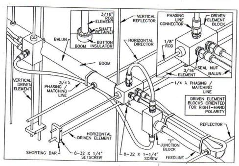
7. Install the 8-32 x 1/4" set screws (internal Allen head - tool supplied) into the SHORTING BARS. Slide the bars onto the 1/8" Driven Element Block Rods and the 3/16" driven element rod. Position the Shorting Bars as specified on the Dimension Sheet: the given distance is between the outer face of the driven element block and the inner face of the shorting bar. Align the bars and rods to each other and tighten the set screws.
