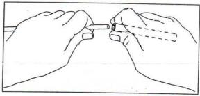
retainer onto the element end and continue until retainer butts on insulator button. Locking pliers, *lightly* clamped up against opposite button insulator will help maintain center reference (if you push the first retainer too far, remove element from boom, push retainer completely off the element, and start over). Install another retainer to the opposite side of the element. Continue installing retainers until all elements are secured.
