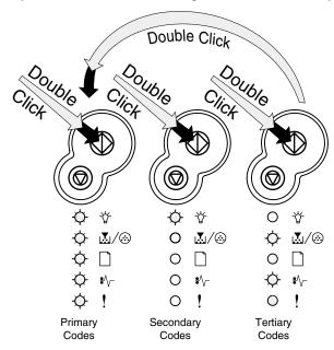
**Note:** All lights flashing simultaneously, as a result of sending data to the printer, may indicate a code problem. Call the next level of support.
