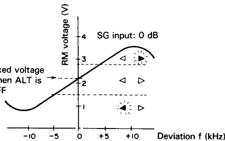
**Fig. 9** Relationship between the RM voltage and deviation during receive
