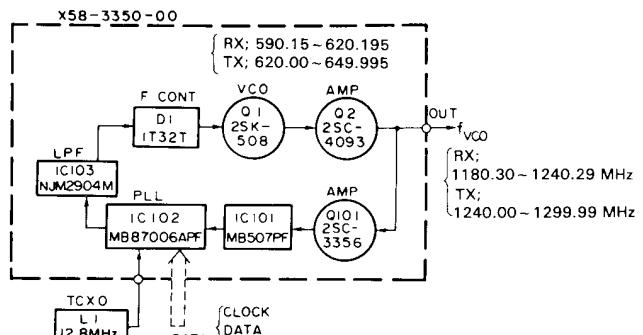
**Fig. 6** Block diagram of the PLL unit
