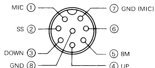
**Fig. 24 MIC terminals (view from front panel side)**
