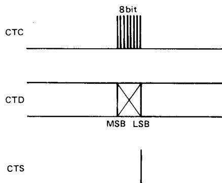
Fig. 22 Transmit form of the CTCSS data
