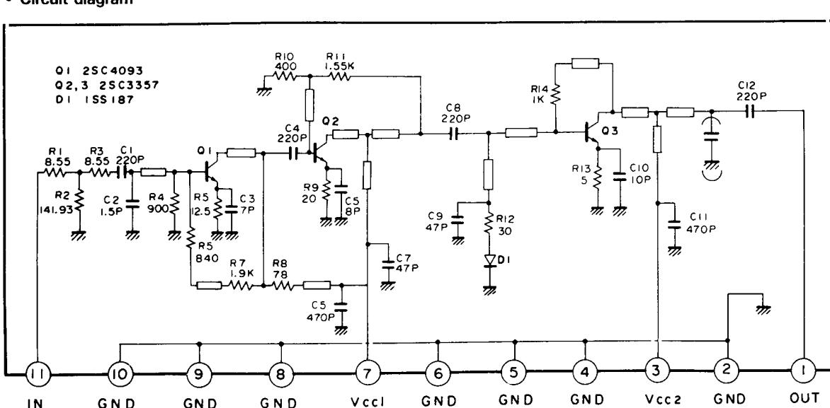
Fig. 11 Circuit diagram of Drive HIC (KCB01)
