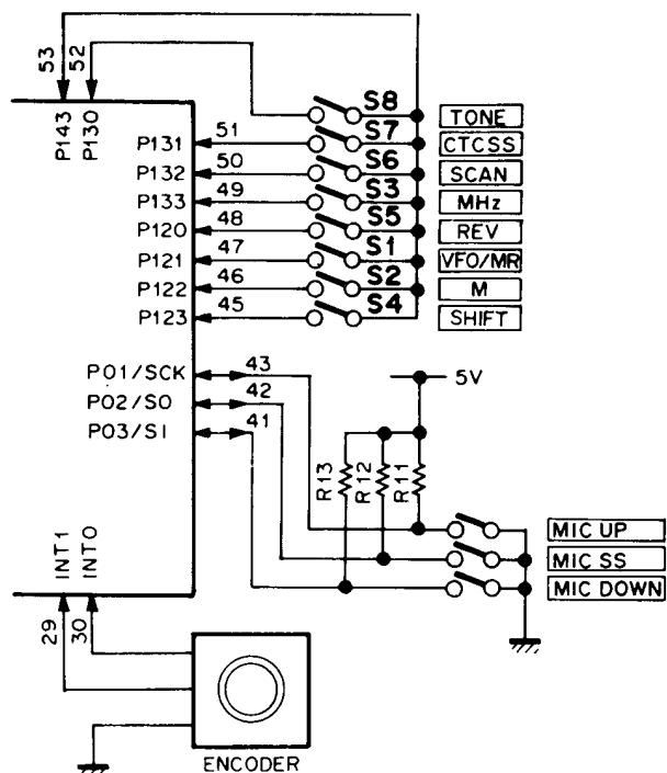
Fig. 12 Key and rotary encoder input circuit
