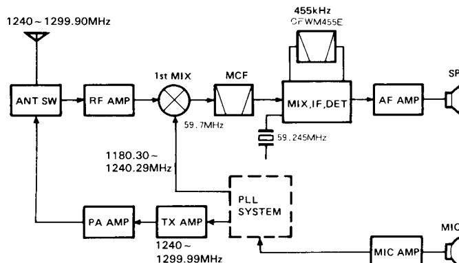
Fig. 1 Frequency configuration diagram
