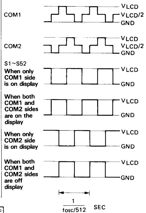
**Fig. 14** Common and segment output signals of the LCD driver
