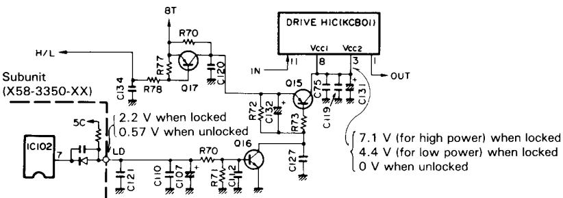
**Fig. 10** Unlock circuit
