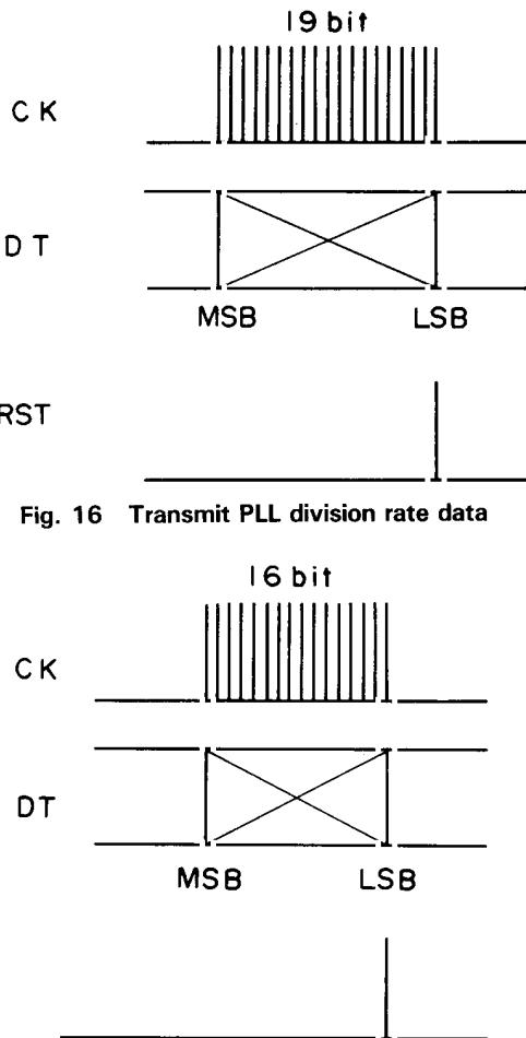
**Fig. 16** Transmit PLL division rate data
