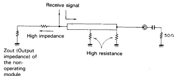
**Fig. 5** Equivalent circuit for receive
