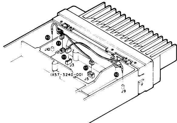
10. Remove the 8 screws (12) that fix the unit to the main chassis, and pull the unit in the direction of the arrow.
