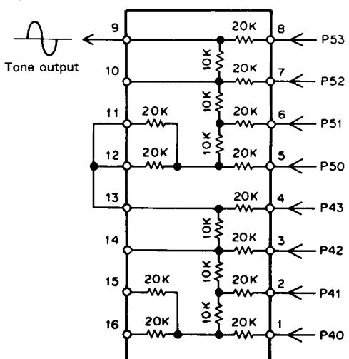
Fig. 21 Ladder resistance network: Control Unit IC4 (KRR-C001)
