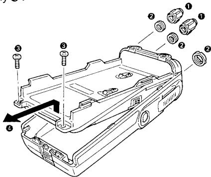
4. Taking care not to cut the speaker lead ⑤, open the chassis and case assembly.
