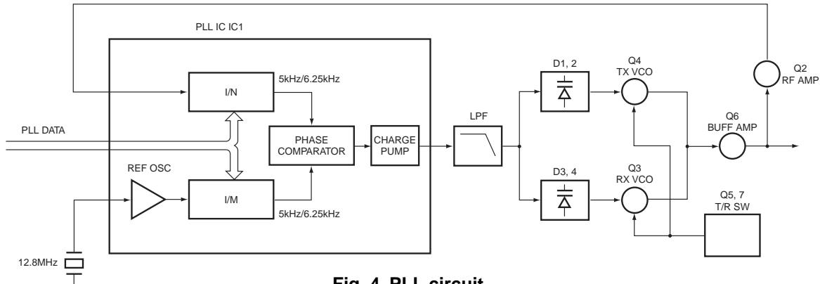
Fig. 4 PLL circuit
