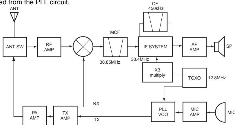
**Fig. 1 Frequency configuration**
