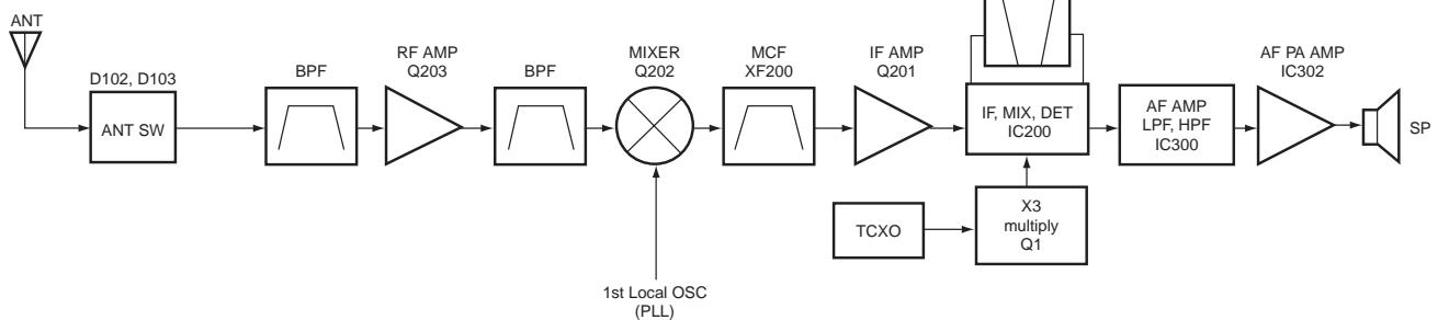
**Fig. 2 Receiver section configuration**
