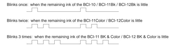
The ink low warning reset function by button operation is added to this printer. The button operation procedures are shown below. (The ink low warning of the BJC-80/80v can be reset from the host computer only.)
